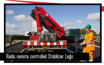
All stabilizer functions (option) can be operated from the remote control box, which is fitted with an HMF InfoCentre. A stabilizer icon appears on the display of the HMF InfoCentre, and it is possible to operate the stabilizer beams and stabilizer cylinders. This makes operation with the stabilizers easier, faster and safer, and the operator has an unobstructed view of all movements.
